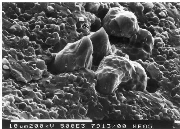
Fig. 8. The fracture surface of a composite containing 5 vol.% Ni inclusions. A plastically deformed Ni inclusion is indicated with an arrow.
